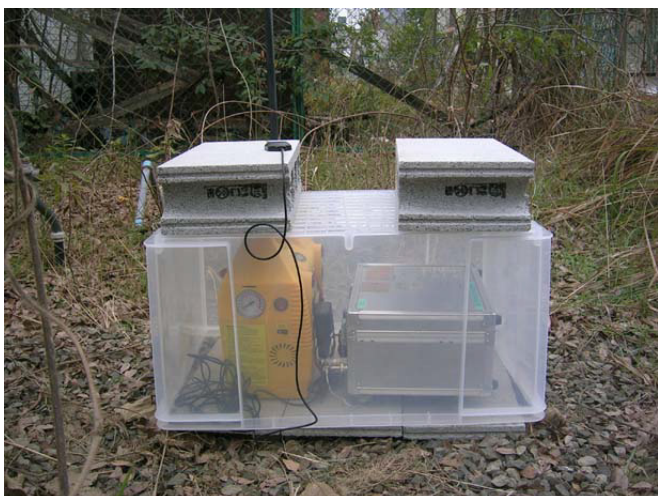
(a) Example of microtremor measurement site (site C)
