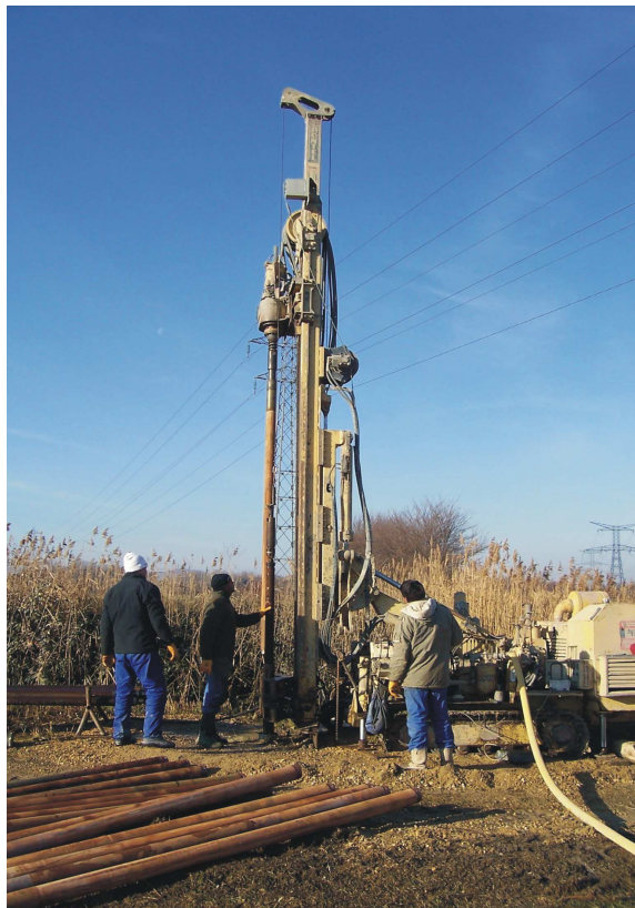
Figure 1 : On the left: drilling operation in preparation to a crosshole measurement, on the right: “PS Suspension Logger” : a diagraphic tool that can generate both P and S waves in the soils (source : www.geovision.com ).
