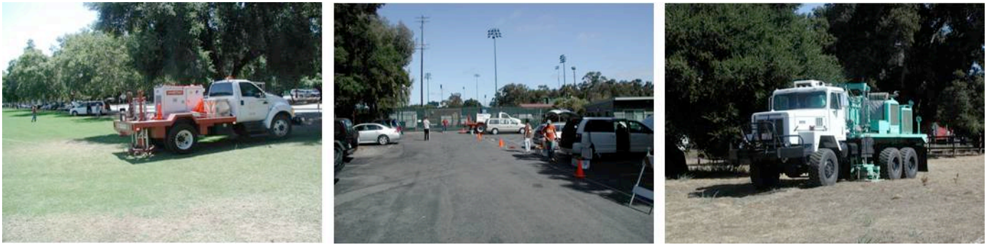
Fig. 3. SASW surveys: (a) Thumper, (b) survey at the Children's Center, and (c) Y1100 vibroseis.
